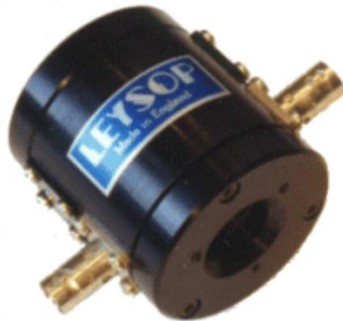
This has a modest half wave voltage (the voltage which must be applied to produce a pi radian phase shift, equal to a polarisation rotation of  $90^\circ$ ) of around 6kV at 1064nm and has extremely high resistance to laser damage as well as being available in excellent quality crystals of large sizes. For these reasons, all our longitudinal mode Pockels cells are manufactured from >95% deuterated KD\*P.
