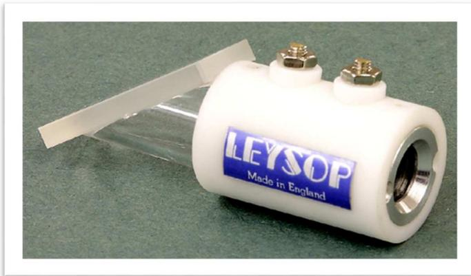
Both the Brewster thin-film polarizer and the low order quarter wave retardation plate will be pre-aligned with the axes of the KD\*P crystal. The standard orientation is for transmitted P=polarization to be parallel to the axis of the connecting studs, but if you prefer we can orientate the studs at 90° to the polarizing optical elements on request.
